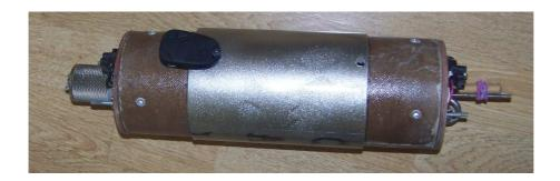
In my rockets what I do is use screw switches to turn on my altimeter so the hole for the screw switch is also used for exchanging pressures.
